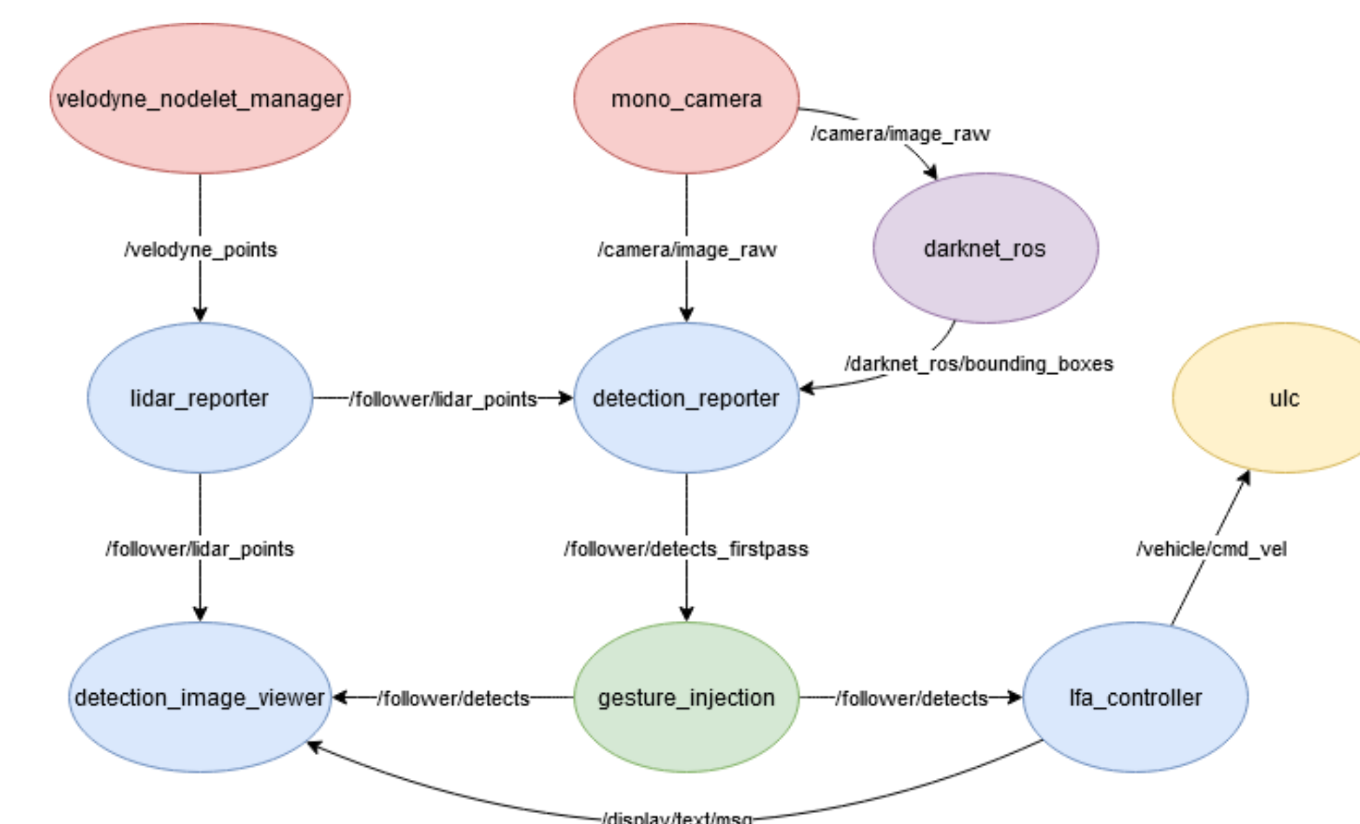
Figure 5: Diagram of ROS node architecture in the SLS
