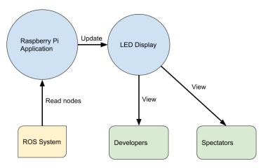
in a separate system from the ROS core the display can continue to display the status of the ROS core even if a fatal error occurs within the ROS core environment.
