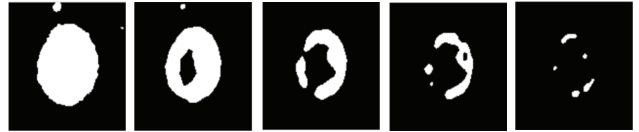
Fig. 2.— Dynamic thresholding binary maps. The Images show binary maps with thresholds of 20 (left), 44, 83, 99, and 115. The figure shows that when using a graylevel of 44 the ring is identified in the binary mask, while other graylevel thresholds show no ring.
